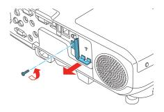
Insert the wireless LAN module into the port.
